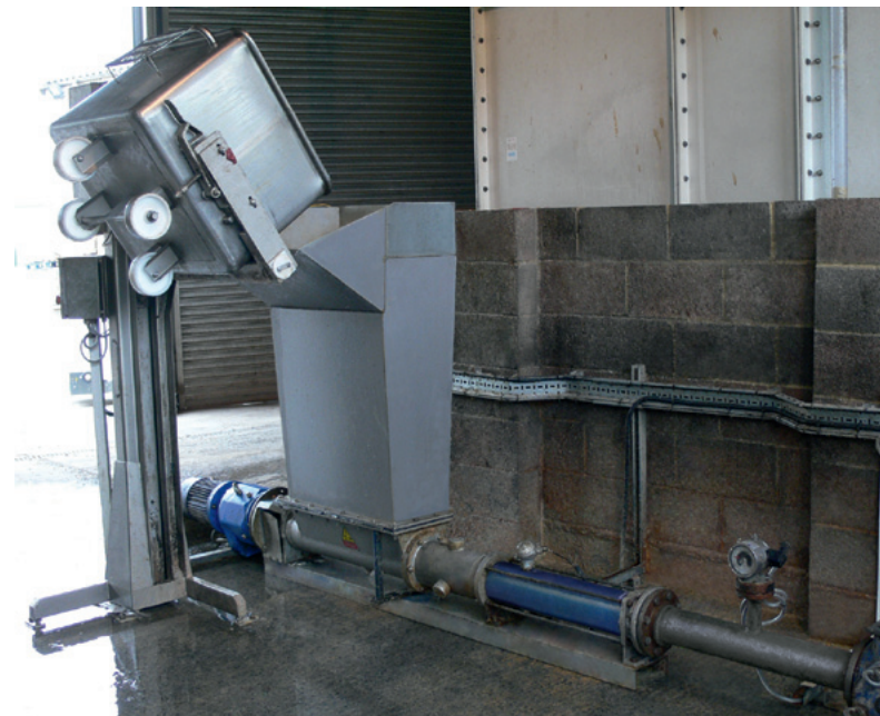
seepex BTM range pump receiving waste from a tote bin
