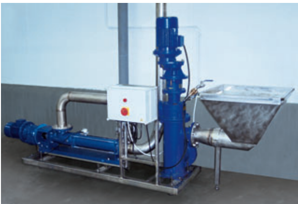
Pump of range BN 10-12 and macerator 25U with solids separator Conveying product: Poultry intestines Conveying capacity: 4 m 3 /h (17 GPM) • Pressure: 6 bar (87 PSI) Temperature: 20 °C (68 °F)
