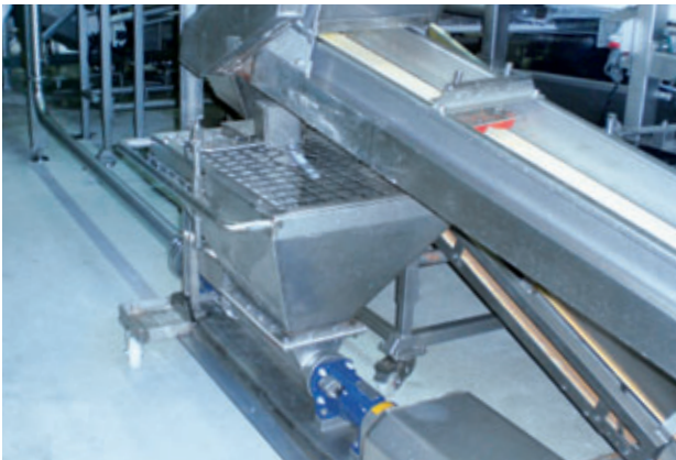
Pump of range TNS 2-12 Conveying product: Unusable diced potatoes from convenience food production Conveying capacity: 1 m 3 /h (4.4 GPM) Pressure: 5 bar (72 PSI) • Temperature: 40 °C (104 °F)
